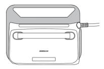
**1.5** Extend the sides and bottom of the teach pendant soft cover to allow the teach pendant to be positioned completely inside the teach p endant soft cover.
