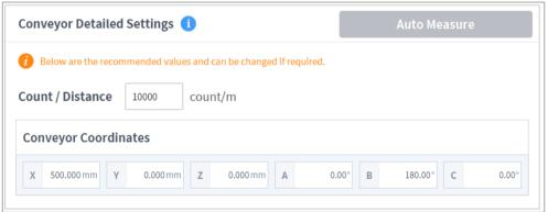
The x-axis of the conveyor coordinates is the direction of the conveyor's movement in terms of the reference coordinates (Base or World).
