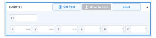
Turn on the conveyor again and stop it in the same way to acquire a location for Point X2. Point X is used to calculate the x-axis of the conveyor coordinates. While just X1 and X2 are sufficient, up to four points can undergo teaching to improve accuracy. Depending on the number of teachings, spread the position within the range where the robot can undergo teaching.
