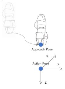
Move to **Action pose**: This is the point on the workpiece where the End Effector performs work. (e.g., Picking Pose, Placing Pose)
