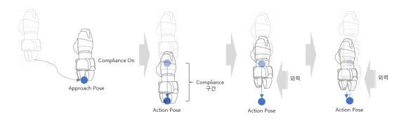
**Contact Check**: The function detects contact with the target, stops at a corresponding position and activates the gripper to grab the target based on the **Contact Force**, **Contact Determination Range** and **Authorized Force** values entered.
