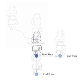
**Move to Action End Pose**: If the End Effector execution target does not end with a single motion, there may be an intermediate point and an end point, and the Action End Pose is the point where the work ends. (e.g., Door Open Skill – End Pose, Screw Drive Skill – End Pose)
