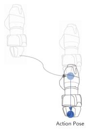
**Move to Retract Pose**: This is the point to pick up the workpiece and move it safely to another point. It is the –Z direction from the approach pose, but a different direction can also be selected. The Retract Distance entered is automatically calculated for the Action Pose and moves to the corresponding point.
