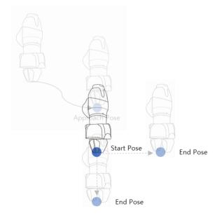
**Move to Action End Pose**: If the End Effector execution target does not end with a single motion, there may be an intermediate point and an end point, and the Action End Pose is the point where the work ends. (e.g., Door Open Skill – End Pose, Screw Drive Skill – End Pose)
