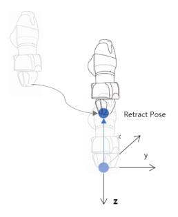
**Move to Action Start Pose**: If the End Effector execution target does not end with a single motion, there may be an intermediate point and an end point, and the Action Start Pose is the point where the work starts. (e.g., Door Open Skill - Start Pose, Screw Drive Skill – Start Pose)
