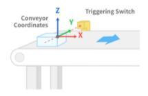
Methods to calculate these values are Auto Measure, after teaching the conveyor teaching points to the robot, and Manual Calculation from the system design specifications. It is possible to use Manual Calculation if it is difficult to teach the robot about the workpiece, but Auto Measure is recommended in most scenarios.
