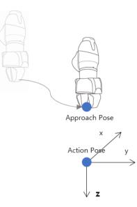
Move to **Action pose**: This is the point on the workpiece where the End Effector performs work. (e.g., Picking Pose, Placing Pose)
