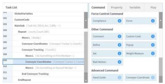
Note that it is necessary to differentiate the first coordinates and the second coordinates when teaching. Select coordinates suited for the workpiece, perform Start Teaching, and perform Get Pose to obtain teaching points suited for each coordinate. If the workpiece is identical, it is acceptable to share identical teaching points.
