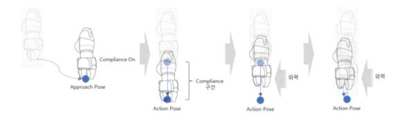
Contact Check: Based on the Contact Force, Contact Determination Range and Authorized Force values entered, the function detects contact with the target, stops at a corresponding position and activates the gripper to grab the target.
