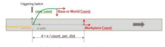
d: distance from conv. coord to workpiece e: incremental encoder value after triggering switch activated
