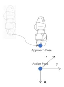
Move to **Action pose**: This is the point on the workpiece where the End Effector performs work. (i.e., Picking Pose, Placing Pose)
