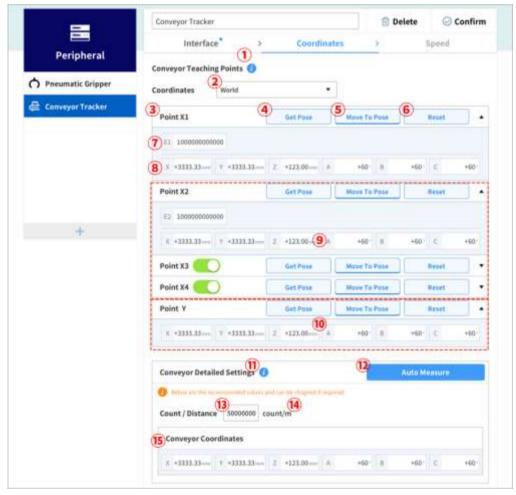
The purpose of the Coordinates tab is to set the Count/Distance value and Conveyor Coordinates of Conveyor Detailed Settings. It calculates the converted value, which indicates how much the Encoder
