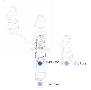
**Move to Action End Pose**: If the End Effector execution target does not end with a single motion, there may be an intermediate point and an end point, and the Action End Pose is the point where the work ends. (i.e. Door Open Skill – End Pose, Screw Drive Skill – End Pose)
