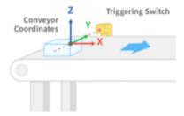
Methods to calculate these values are Auto Measure after teaching the Conveyor Teaching Point to the robot and Manual calculation from the system design specification. Auto Measure is recommended for the purpose of reducing errors, but Manual calculation is possible of it is difficult to teach the robot of the workpiece.
