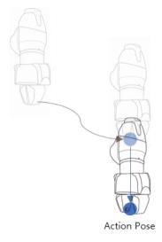
**Move to Retract Pose**: This is the point to pick up the workpiece and safely move to another point. It is the -Z direction from the Approach Pose, and a different direction can also be selected. The Retract Distance entered is automatically calculated for the Action Pose and moves to the corresponding point.
