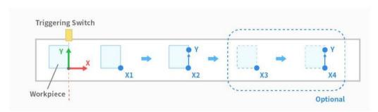
Place a workpiece on the conveyor in the same way it would be during actual work. Operate the conveyor and stop the conveyor as soon as the workpiece passes the triggering switch of the conveyor. Teach the reference point of the workpiece at this moment, and acquire the location of Point X1 using Get Pose.
