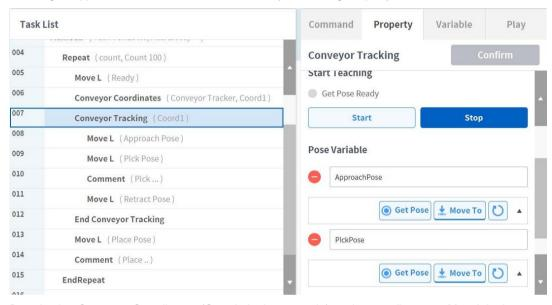
By selecting Conveyor Coordinates (Coord1 in the example) as the coordinates at MoveL in the Conveyor Tracking node, it is possible view teaching points that underwent teaching at Conveyor Tracking. Select a teaching point (ApproachPose, PickPose) to complete programming.
