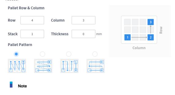
To automatically calculate the offset direction of stacked or picked items according to the pallet's upward/downward direction, it is recommended that the Workcell item's three points be instructed in a counter-clockwise direction on a guide image.
