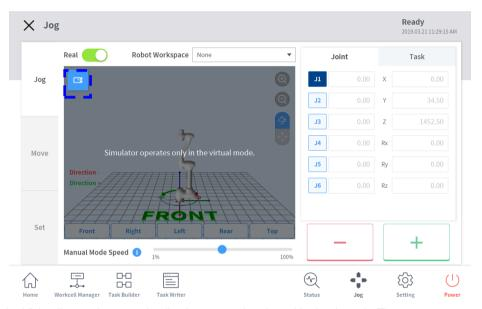
If the Vision license is entered, a live image can be viewed in the Jog tab. The user can operate the robot while viewing the live image.
