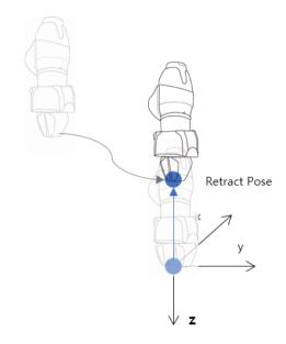
**Move to Action Start Pose**: If the End Effector execution target does not end with a single motion, there may be an intermediate point and an end point, and the Action Start Pose is the point where the work starts. (i.e. Door Open Skill - Start Pose, Screw Drive Skill - Start Pose)
