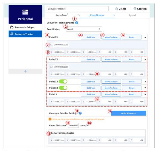
The purpose of the Coordinates tab is to set the Count/Distance value and Conveyor Coordinates of Conveyor Detailed Settings. It calculates the converted value, which indicates how much the Encoder Count increases when the conveyor moves, and which point the conveyor is fixed to in a particular space. The x-axis of the Conveyor Coordinates is the direction the conveyor moves in terms of the reference coordinates (Base or World).
