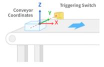
Methods to calculate these values are Auto Measure after teaching the Conveyor Teaching Point to the robot and Manual calculation from the system design specifications. Auto Measure is recommended for the purpose of reducing errors, but Manual calculation is possible if it is difficult to teach the robot of the workpiece.
