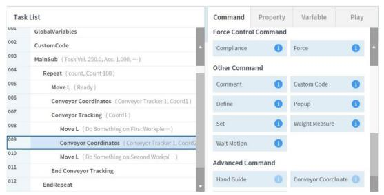
Note that it is necessary to differentiate the first coordinates and the second coordinates when teaching. Select coordinates suited for the workpiece, perform Start Teaching, and perform Get Pose to obtain teaching points suited for each coordinate. If the workpiece is identical, it is acceptable to share identical teaching points.
