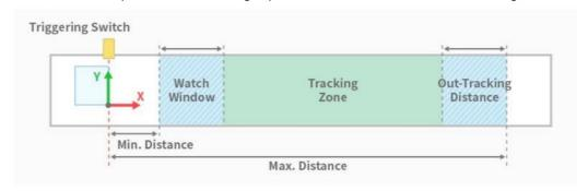
The Watch Window in the Conveyor Section is the area that determines work candidates. Workpieces in this area can only be targets once the work begins. The work itself can begin with the Watch Window, but in the worst case, this can cause workpiece at the end of the Watch Window to be a target, so it is recommended to adjust the Watch Window size to allow all work in the Tracking Zone to be completed.
