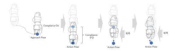
**Contact Check**: The function detects contact with the target, stops at a corresponding position and activates the gripper to grab the target based on the **Contact Force**, **Contact Determination Range** and **Authorized Force** values entered.
